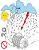
Check that all the gaskets are in perfect condition and well seated in their places; check that the cable inlet openings are properly closed so that the IP protection degree shown on the motor plate is respected.
