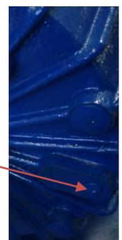
When the two plugs are removed screw the two brake release screws (131).
