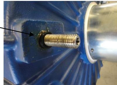
To reassemble the brake hand release proceed backwards. When mounting the unlocking hand brake lever (128), be sure to leave an airgap between the lever and the brake cover.
