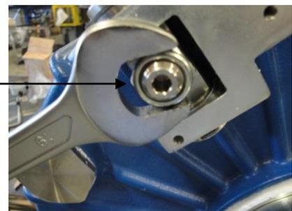
Take the unlocking hand brake lever (128) off the hand brake release screws (118).
